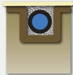
Sandtrapper II, MD and I are all able to be placed over drainage lines. By doing so, maximum performance against drainage gravel contamination is achieved.
